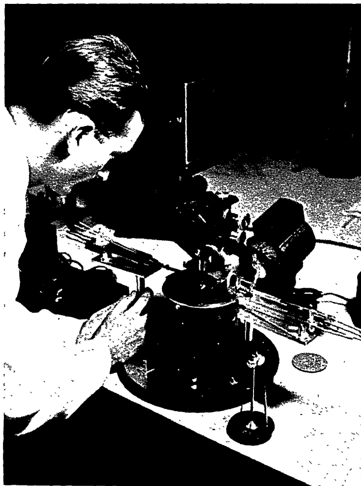
This illustrates the type of apparatus used in modern micrurgical research. Injections and manipulations of microscopic specimens can be performed with instruments of this kind. This was taken in the Division of Micrurgical Research.
