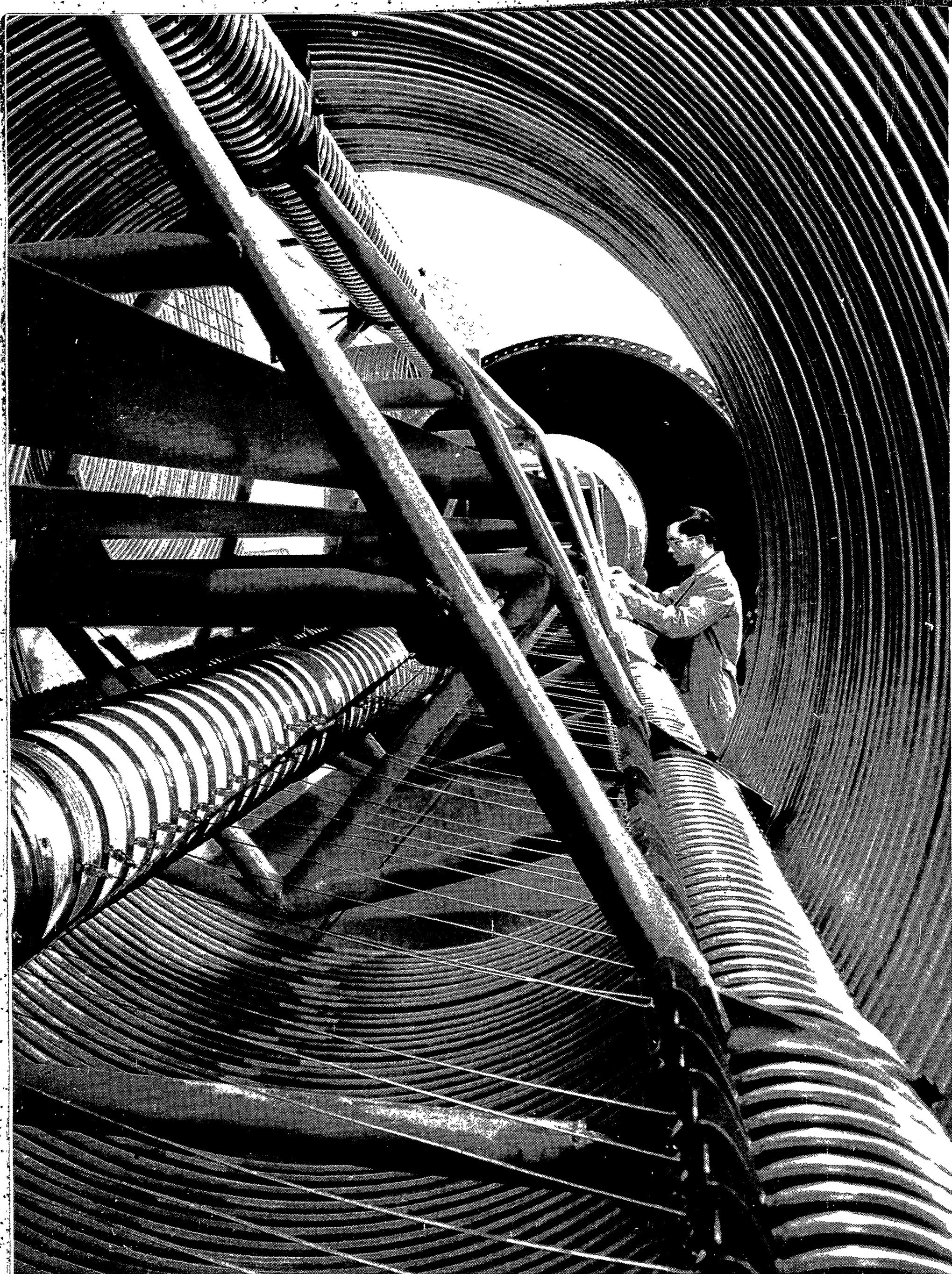
Notre Dame's atom smasher, located in Science Hall. Weighing 50 tons this generator is 40 feet long and 8 feet in diameter. The 202 aluminum hoops distribute charges uniformly and prevent sparking.
